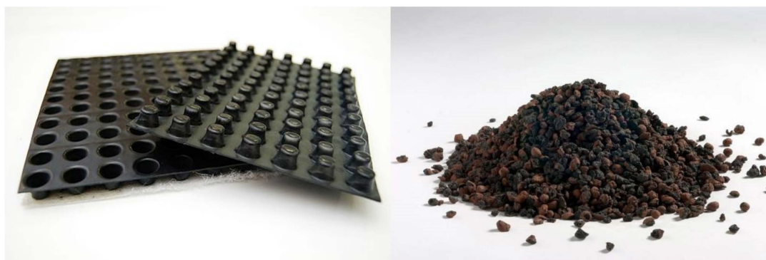
Figure 2. Green roof drainage materials: Modular panels (on the left) and granular materials (on the right).
